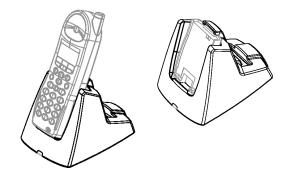
The Companion Individual Charger can charge a handset or a spare battery pack. To charge a separate battery pack in the desktop charger, you must place the battery pack under the tab in the desktop charger.
